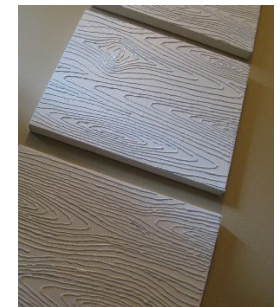
Faux wood grain is an inappropriate finish in the historic district because it does not present an authentic appearance.
